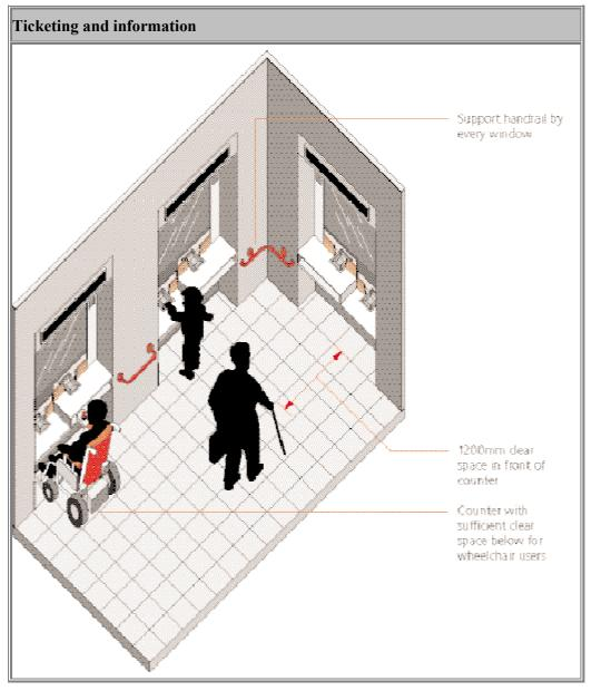
The design of the counter top is also important. Some counters have a large radius curve on the top leading edge and when a customer sweeps the change or ticket into their hand it falls to the floor. A slight upstand at the front edge of the counter facilitates picking up small items. The design of the counter top should also reduce glare and reflection from lighting both natural and artificial.
