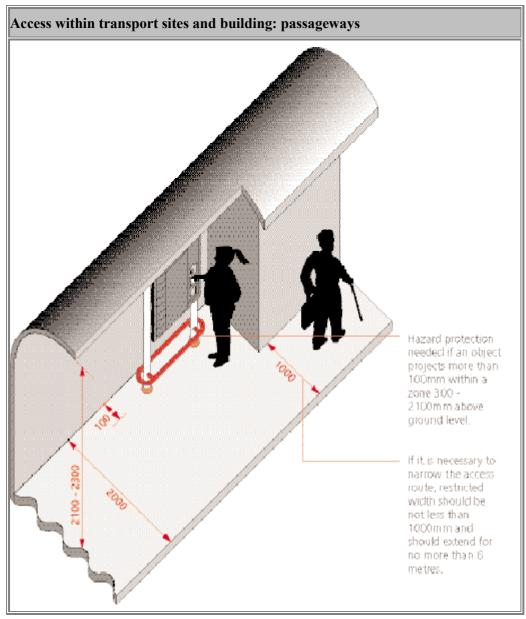
Where it is necessary to introduce occasional narrowing of the access route, the restricted width should not be less than 1000mm and should extend for no more than 6 metres.
