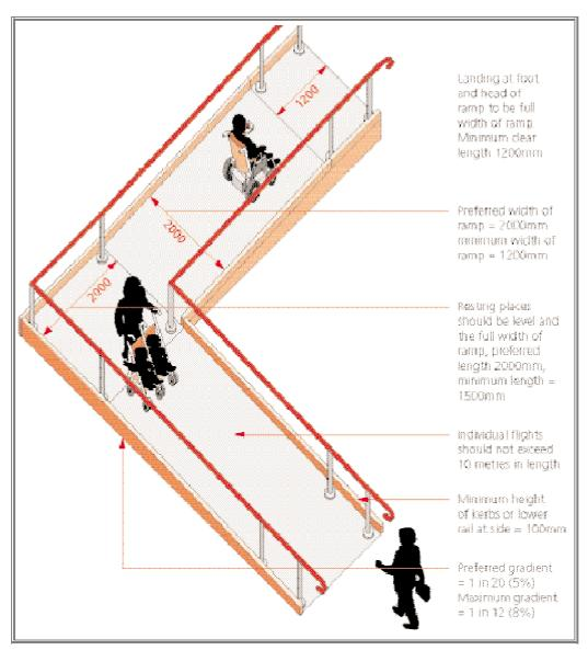
As described in Section 3.2, most guidelines specify **5 per cent (1 in 20)** as the preferred gradient and **8 per cent (1 in 12)** as the absolute maximum acceptable. There is a relationship between the length of a ramp and the gradient that people can manage; the longer the ramp the less severe the gradient that is feasible. One possible approach to this is, where a lengthy ramp is necessary, to design more frequent landings and lesser slopes for each successive segment.
