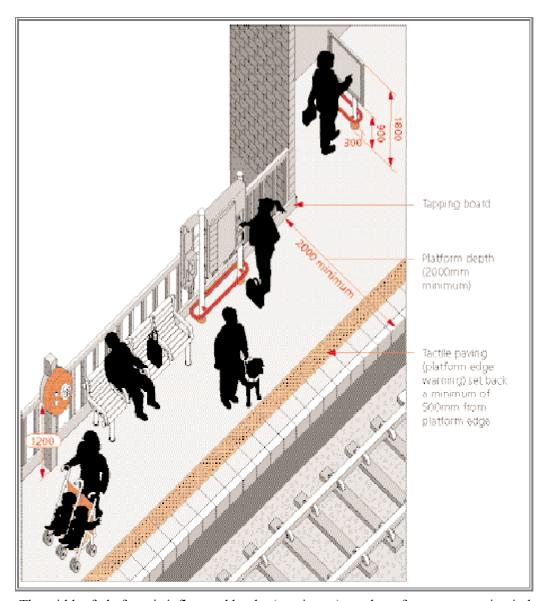
The width of platform is influenced by the (maximum) number of passengers using it, but should have a minimum of **2000mm** clear space in addition to the width of the safety zone(s) and a further **1000mm** for service traffic.
